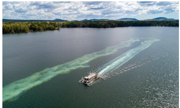
A large barge is used to add alum to lakes with chronic internal P loading. (Photo credit, Georges Pond Association)
